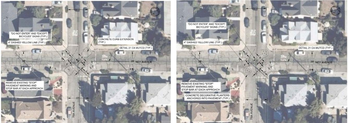
Figure 20. Ney Avenue at 75th Avenue diagonal diverter concrete and planter options
