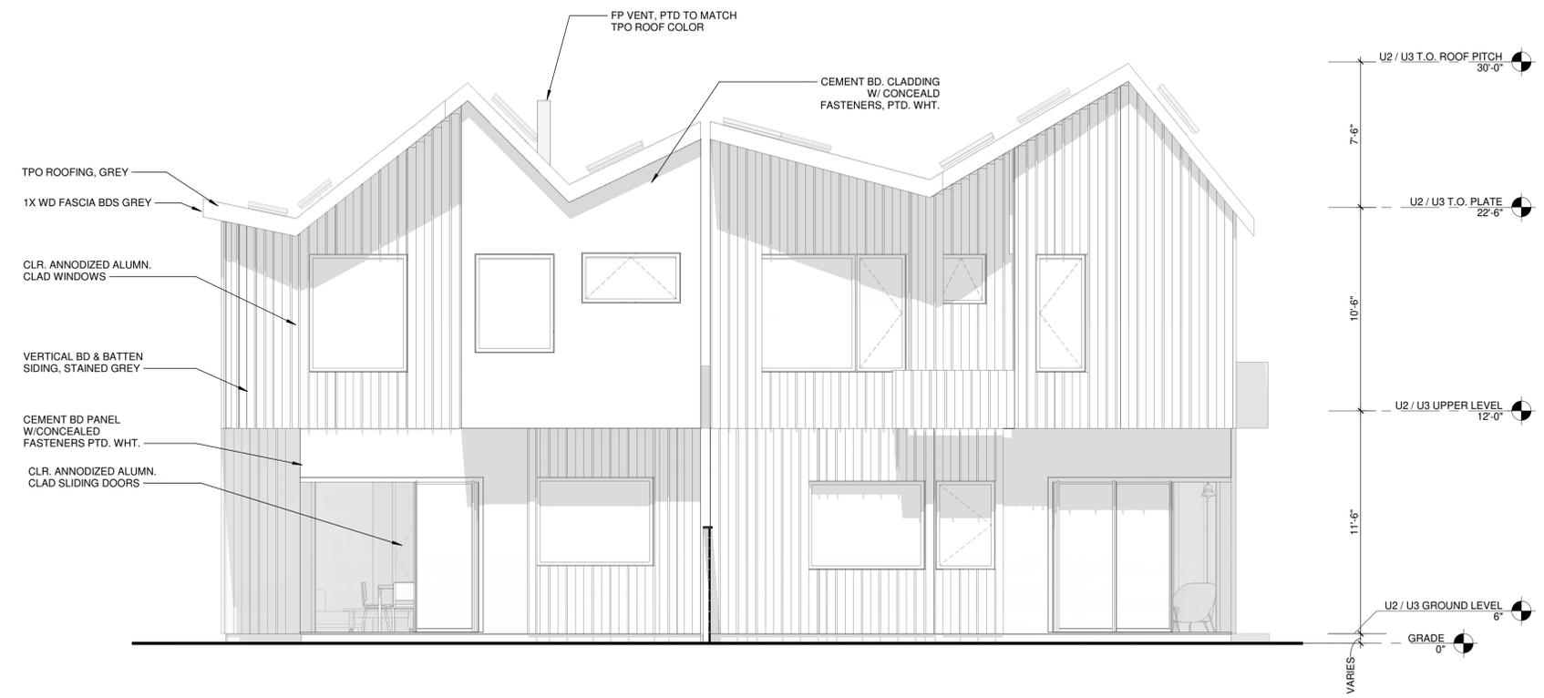
**2 SOUTH ELEVATION - UNIT 2 / UNIT 3**
