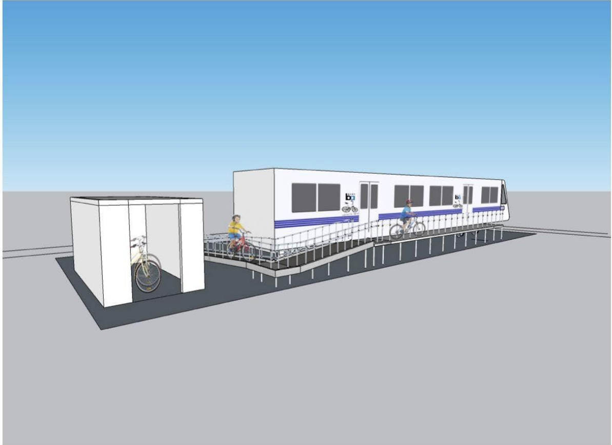
Rear access through an ADA-compliant ramp
