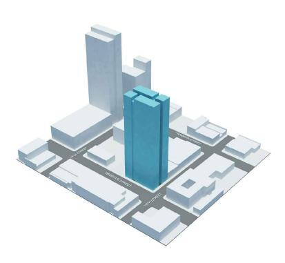
2: CUT MASS INTO TWO BARS. ADD BALCONIES TO THE MIDDLE VOID. ADD A VERTICAL RECESS UP THE EAST AND WEST ELEVATION.
