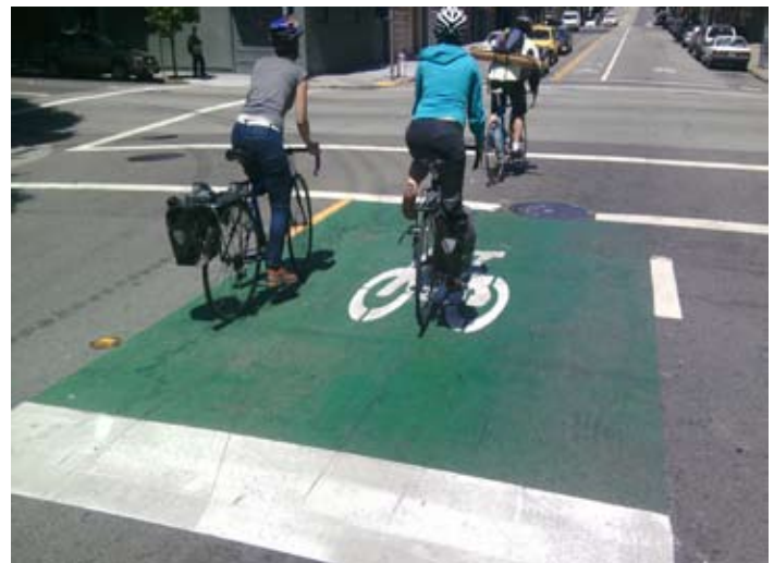
“Bike Box” Bicycle Facility, San Francisco, CA
