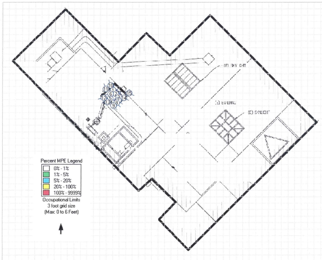
Plot #1: Ground level. The plot shows the maximum predicted power density levels between 0 and 6 feet above the ground as a percentage of the Occupational Limit.
