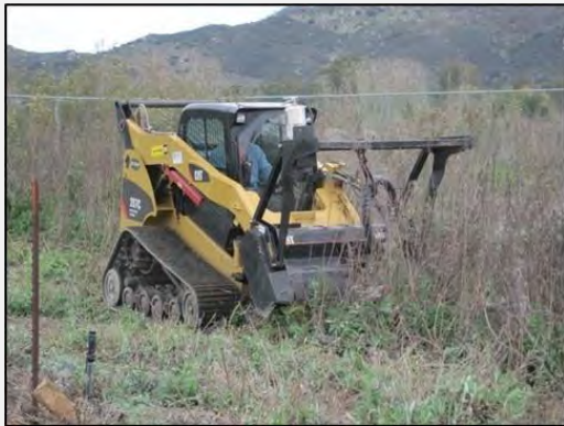
Exhibit 8. Masticator attachment on a bobcat.
