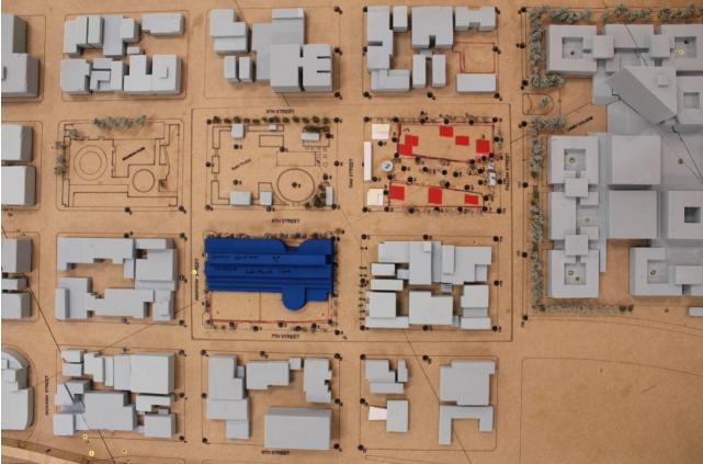
Image 2A: Wind Tunnel Study Model – Existing Configuration
