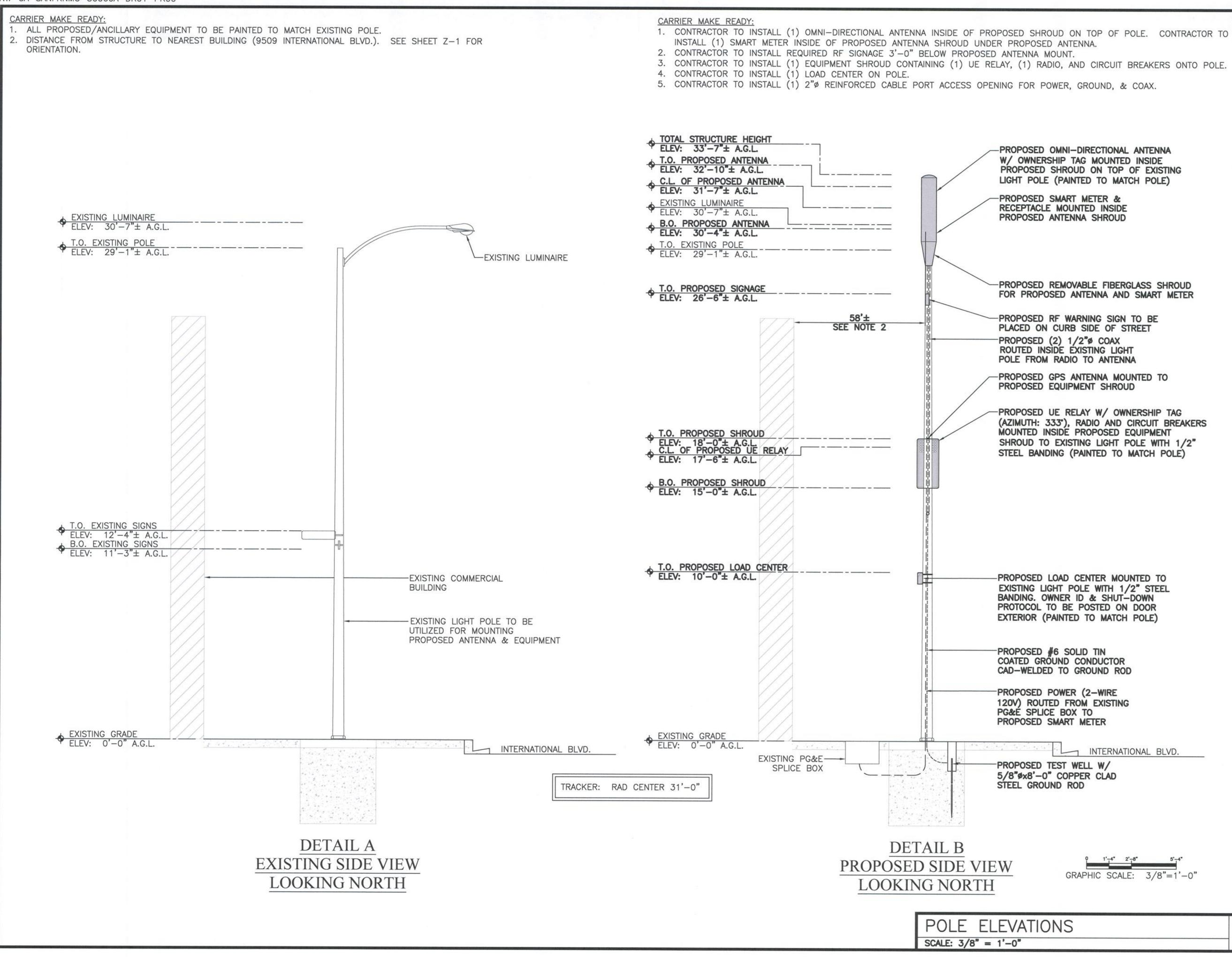
PROPOSED OMNI-DIRECTIONAL ANTENNA W/ OWNERSHIP TAG MOUNTED INSIDE PROPOSED SHROUD ON TOP OF EXISTING LIGHT POLE (PAINTED TO MATCH POLE)
