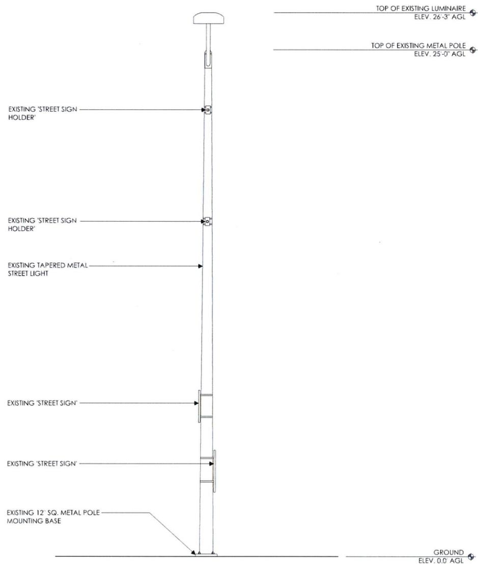
**SOUTH ELEVATION - EXISTING**
