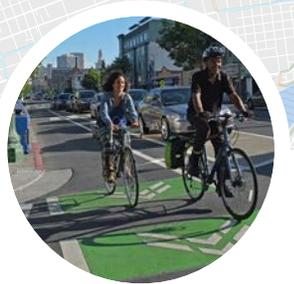
**2** Oakland's first parking protected bikeway on Telegraph Ave has illustrated the safety benefits of increased separation - with a 40% reduction in collisions measured after installation.
