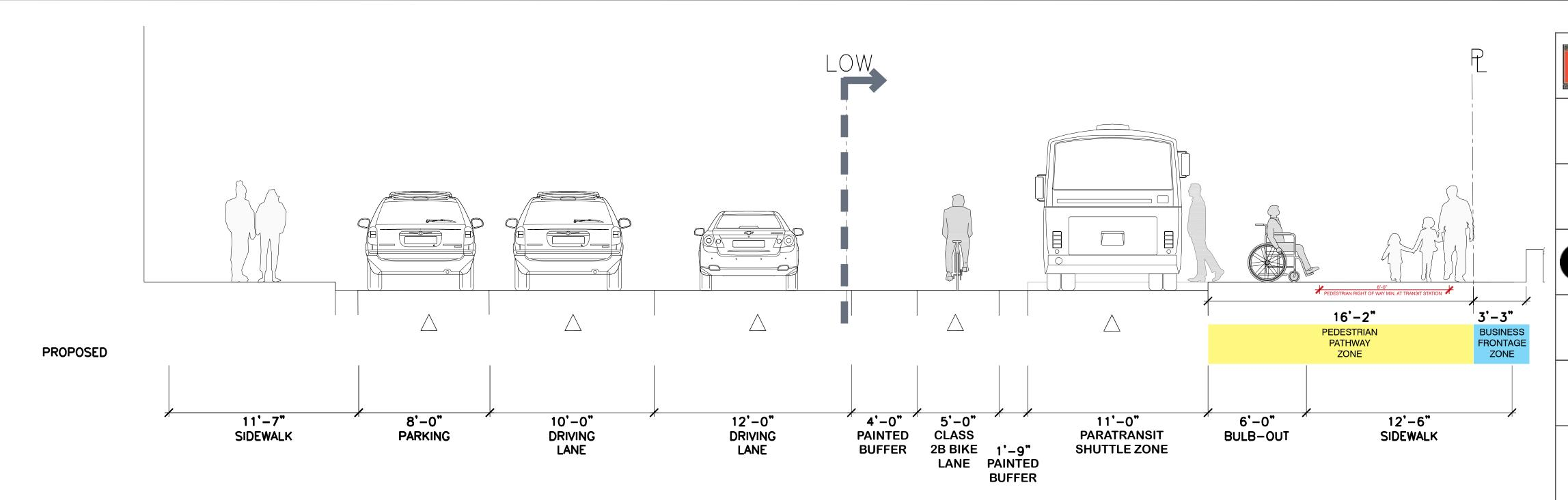
**Typical Cross Section: A Shuttle Zone**
