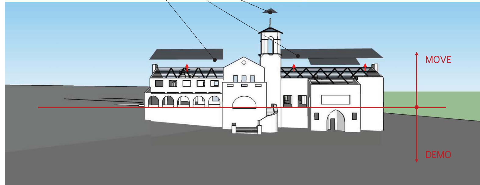
5 DEMO ROOF SHEATHING / RECYLCE DEMO
