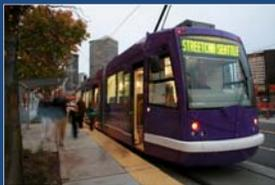
Streetcars are a highly-localized, low-impact form of rail transit which run in mixed-traffic flow powered by an overhead wire.
