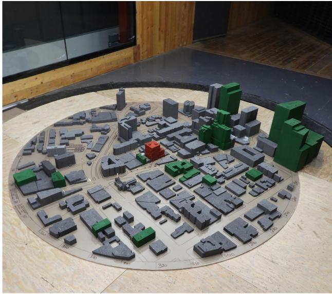
Image 2C: Wind Tunnel Study Model – Project + Cumulative Configuration
